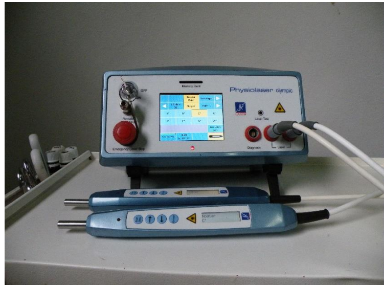
Abb. 1, links: Laserpen 70mW 785nm, Fa. Reimers&Janssen, Berlin, Abb.2, rechts: Physiolaser 2x90 Watt 904nm Impulslaser, Fa. Reimers &Janssen, Berlin.
