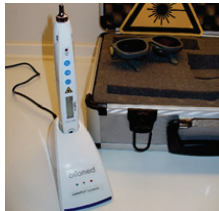
Figure 2: Laser Pen 40 W/904nm for acupoint stimulation in charging station.
